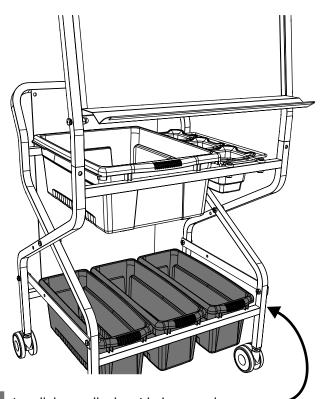
Install the small tubs with the curved front handles pointing to the front of unit.
