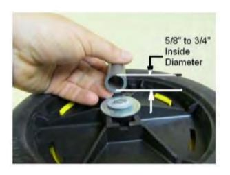
Step 10: Gently tap the end of the Pipe/Socket forcing the Lock Washer onto the end of the axle. DO NOT drive the Lock Washer too far onto the axle and check often to make sure that this is not happening. Refer to Step 11 for further description.
