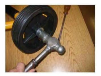
Step 5: Place the washer that is supplied onto the axle, then place the wheel onto the axle in the order as shown.
