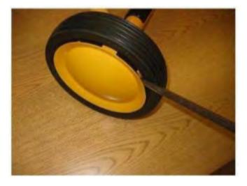
Step 4: Gently tap the end of the axle with the hammer to position the axle correctly.
