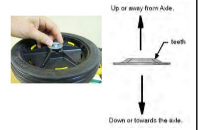
Step 9: Place a piece of pipe, or socket, with the dimension shown on top of the Lock Washer.
