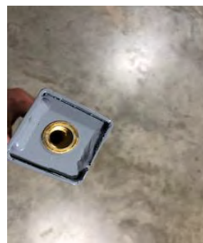
Step 5: Attach threaded caster to leg insert. Tighten with ¾" wrench. Continue until all 4 casters are tight.
