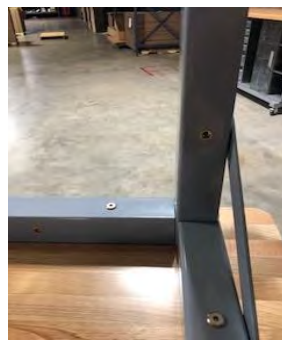
Step 4: Attach brace plate to leg and frame using ¼-20 x 20mm serrated bolts. 2 plates per leg, 8 total.
