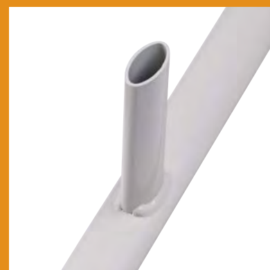
Elliptical tubing depth section is twice as thick as in round tubing. Passes ANSI/BIFMA tests for back strength, back durability, seating drop, seating impact, leg strength and tablet arm load.
