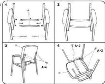
Insert and loosely tighten all screws. When assembly is completed, fully tighten all screws before using. This chair is only intended for sitting. Any other use will void the warranty.
