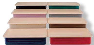
**Bookbox:** Open front: 4-1/2" x 22" x 15" deep, 20-gauge, One Piece, seamless, deep drawn steel box. Die formed pencil groove. Embossed for minimum vibration and maximum strength. Bookbox is riveted to frame at five points.
