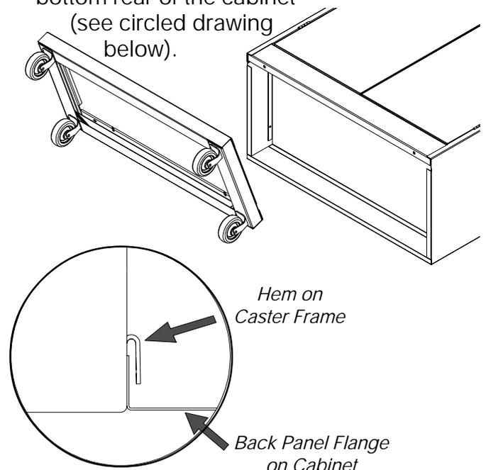
6. Secure the cabinet to the caster kit frame by attaching at the front with two  $\frac{5}{16}$ "-18 x  $\frac{3}{4}$ " bolts and nuts (Ref. Nos. 4 and 5) through the sill as shown. Use a  $\frac{1}{2}$ " wrench to tighten securely.
