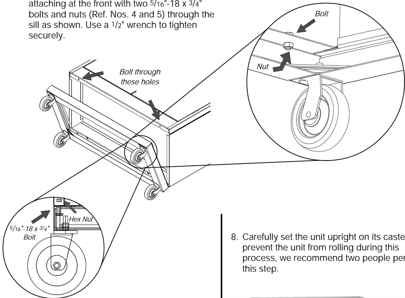
7. Before setting the storage cabinet upright, be sure that all bolts and nuts are tight and that the frame is secure.
