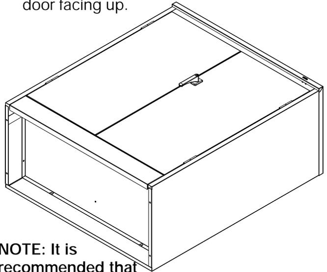
**NOTE: It is recommended that the bottom of the cabinet is a minimum of  $\frac{1}{2}$ " off the floor, in order to more easily attach the caster kit to the unit.**
