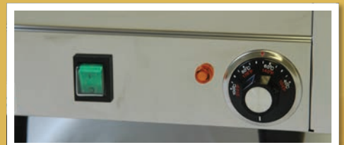
Covered master switch and adjustable thermostat
