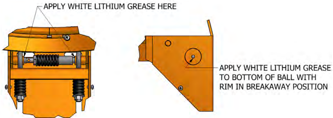
Figure 7-1: Lubrication locations.
