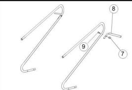
2. Using a wrench and the supplied Allen wrench, attach four handles (part #8) to main racks with four socket screws (part #9)
